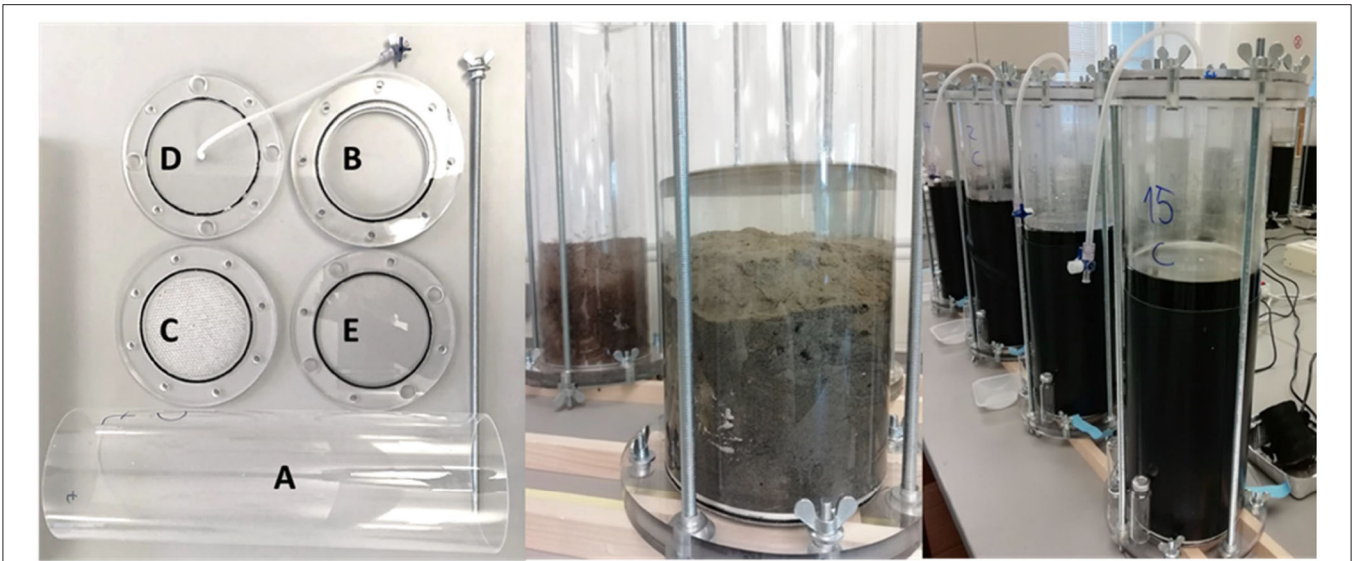
FIGURE 1 | Mesocosm apparatus. Each mesocosms consisted of one fixed part and one removable part. The fixed part consisted of a cylinder ( h = 485 mm, outer/inner d = 150/142 mm; A) attached to an open plate at the top ( d = 210 mm, t = 20 mm; B) and to a perforated plate at the bottom ( d = 210 mm, t = 12 mm; C). Plates B and C had an indentation fitted with a rubber gasket, to ensure that all 3 parts were sealed tightly. The removable part consisted of 2 plates, a top plate and a bottom plate ( d = 210 mm, s = 8 mm, D and E, respectively). Plates D and E were fitted with a rubber gasket, to ensure that all parts (A–D) were sealed tightly during deployment for the gas measurements. Plate D was equipped with the gas sampling apparatus, and was attached to plate B during gas sampling. Plate E was secured to plate C and was removed when the test mesocosms needed to be drained. All mesocosms parts were attached together with lengthwise bolts, screws, nuts, butterfly nuts and washers. The mesocosms were covered with a solid black liner to prevent light exposure.
