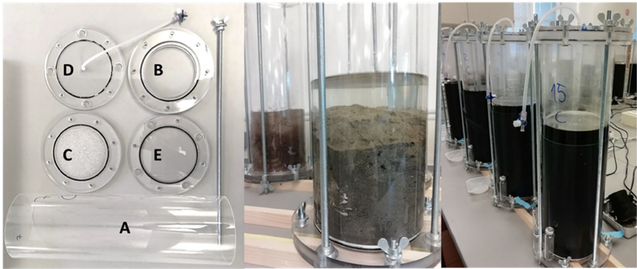
FIGURE 1 | Mesocosm apparatus. Each mesocosms consisted of one fixed part and one removable part. The fixed part consisted of a cylinder ( h = 485 mm, outer/inner d = 150/142 mm; A) attached to an open plate at the top ( d = 210 mm, t = 20 mm; B) and to a perforated plate at the bottom ( d = 210 mm, t = 12 mm; C). Plates B and C had an indentation fitted with a rubber gasket, to ensure that all 3 parts were sealed tightly. The removable part consisted of 2 plates, a top plate and a bottom plate ( d = 210 mm, s = 8 mm, D and E, respectively). Plates D and E were fitted with a rubber gasket, to ensure that all parts (A–D) were sealed tightly during deployment for the gas measurements. Plate D was equipped with the gas sampling apparatus, and was attached to plate B during gas sampling. Plate E was secured to plate C and was removed when the test mesocosms needed to be drained. All mesocosms parts were attached together with lengthwise bolts, screws, nuts, butterfly nuts and washers. The mesocosms were covered with a solid black liner to prevent light exposure.
