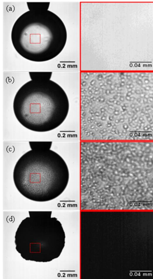
Figure 1. Left: Pictures ( $1 \times 1 \text{ mm}^2$ ) of a pendant drop for  $[\text{Span } 80] = 10 \text{ g/L}$  at  $30 \text{ }^\circ\text{C}$  and at different times. (a)  $t = 0 \text{ s}$ , (b)  $t = 1100 \text{ s}$  and (c)  $t = 1400 \text{ s}$  and (d)  $t = 10000 \text{ s}$ . Right: Zoom in the selected region of interest (red square in right images).
