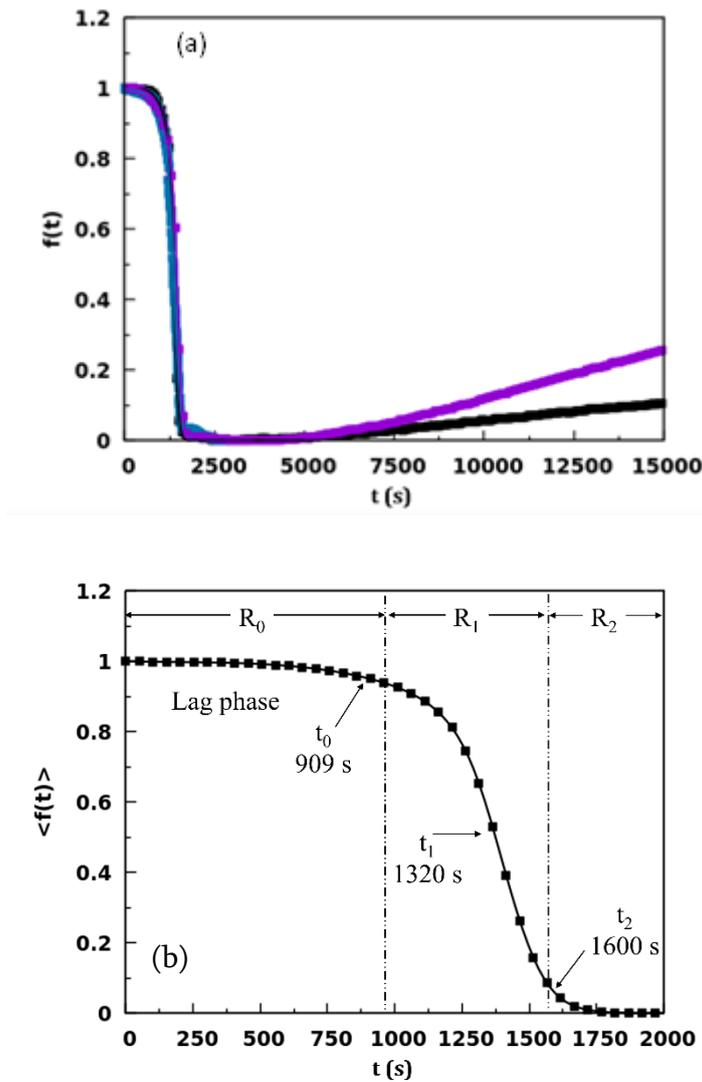
Figure 2. (a): Evolution of  $f(t)$  for  $[\text{Span } 80] = 10 \text{ g/L}$  at  $30^\circ\text{C}$  up to  $t=15000 \text{ s}$  for three identical experiments. Evolution becomes irreproducible once the drop undergoes shrinking ( $t > 2500 \text{ s}$ ). (b): Evolution of averaged fitted contrast function  $\langle f(t) \rangle$  for the three experiments shown in (a) and time sequences associated to regimes  $R_0$ ,  $R_1$  and  $R_2$ .
