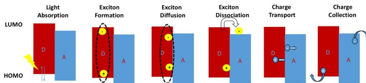
Figure-7: The fundamental steps for the working principle of an OSC.
