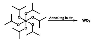
Figure-15: Transformation of tungsten(VI) isopropoxide into WO<sub>3</sub>.
