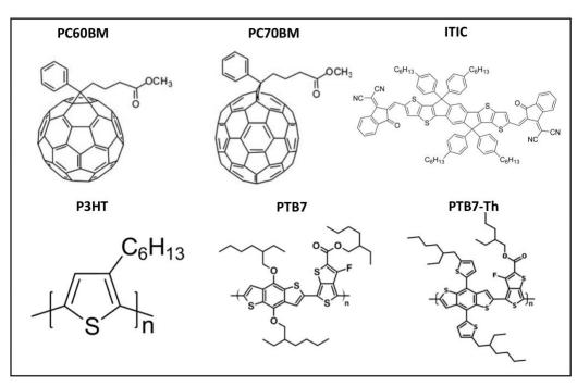
Figure-2: Chemical structures of some donors and acceptors used in OSCs.
