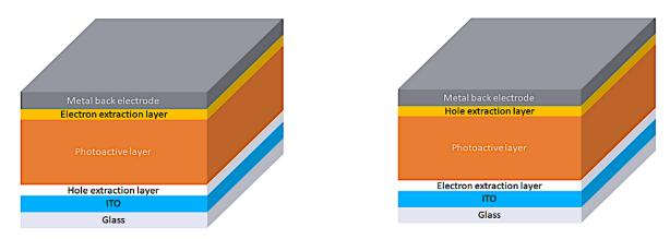
Figure-3: Typical regular (left) and inverted (right) device structures.
