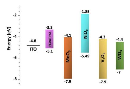
Figure-14: Schematic energy level diagram of typical HTLs used for OSCs.
