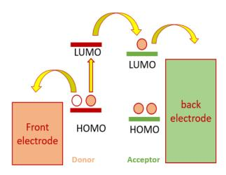
Figure-6: Working principle of organic solar cells.
