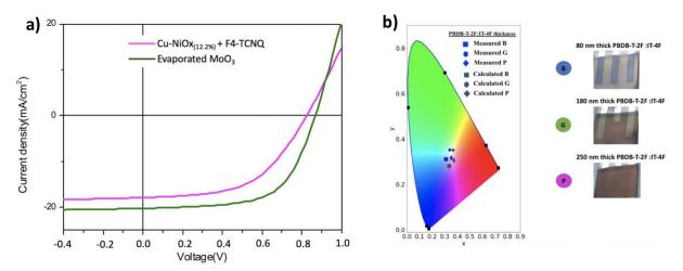
Figure-16: (a) The J–V curves of PBDB-T-2F:IT-4F-based inverted device structures using different HTLs and (b) the color coordinates for the experimental cells (left) along with their photographic images (right). Reproduced from Ref. 134 with permission from the Royal Society of Chemistry.
