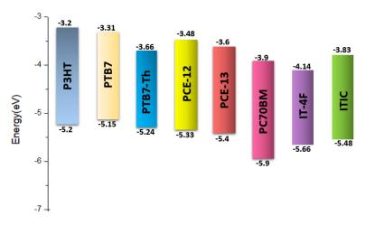
Figure-10: Schematic diagram of the energy levels of some donors and acceptors used for OSCs.
