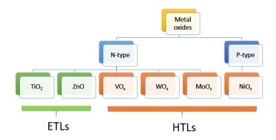
Figure-13: Classification of TMOs into n-type and p-type.
