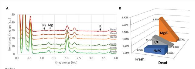
(A) Processed EDX spectra of *E. coli* (Q5586) at the fresh state and after exposure to 70% ethanol. Each curve represents the average of three spectra taken from the same bacterial deposition. Spectra are offset by 3. (B) Evolution of the K/C, Mg/C, and Na/C ratios between the fresh and the alcohol-killed *E. coli*.
