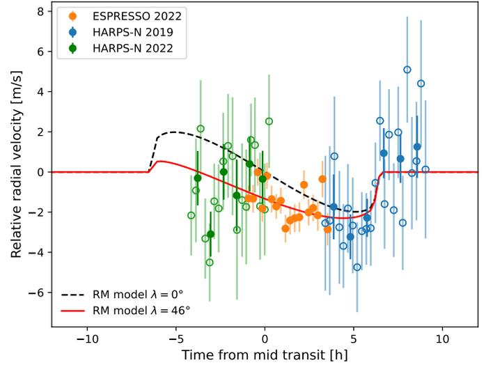
**Fig. 1.** RM effect for HIP41378 d. For HARPS-N 2019 (blue) and HARPS-N 2022 (green), the empty circles are the data used for the analysis, and the filled circles are the binned data. The red line is the best fit from the combined RM effect and a GP which has a projected obliquity of  $\lambda = 46^\circ$ . The dashed black line is the same model with a projected obliquity of  $\lambda = 0^\circ$ .
