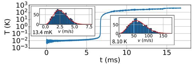
FIG. 1. Temperature evolution of a 1024 ion ensemble, in a trap defined by  $q_x = 0.64$  and  $\omega_z/2\pi = 388$  kHz. The temperature is computed following Eq. (4). The two insets show the velocity distribution of a 1024 ion ensemble at 13.4 mK and 8.10 K as histogram. The red curve is the computed Maxwell-Boltzmann distribution at this given temperature.
