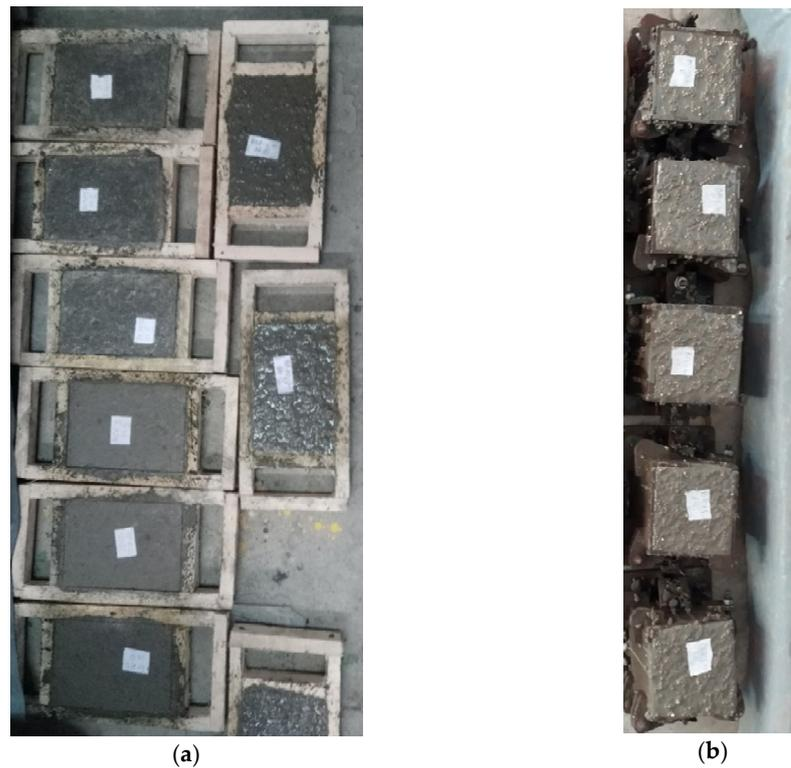
**Figure 4.** View of concrete samples: (a) cubic shape concrete samples, (b) plate shape concrete samples.
