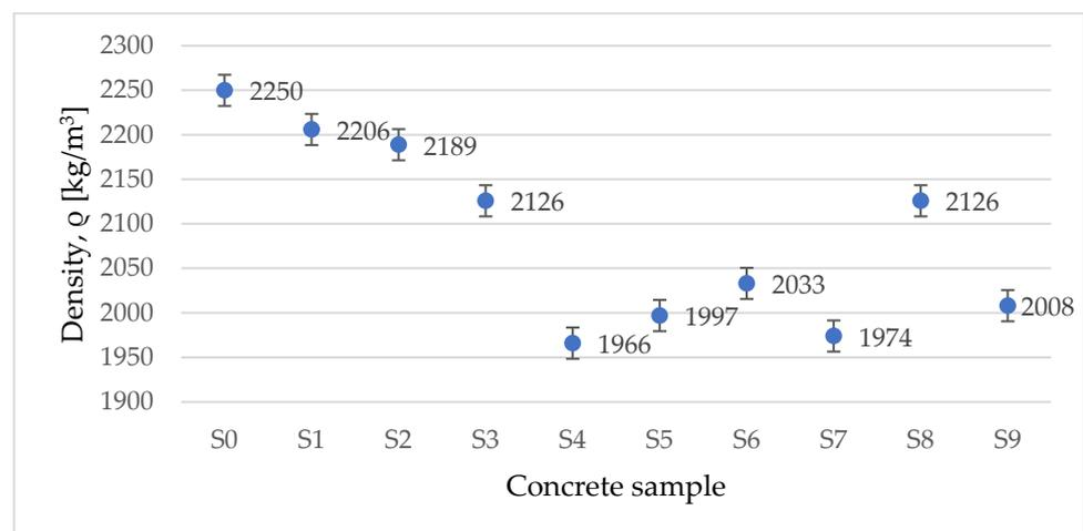
**Figure 6.** Variation of density for tested concrete samples.
