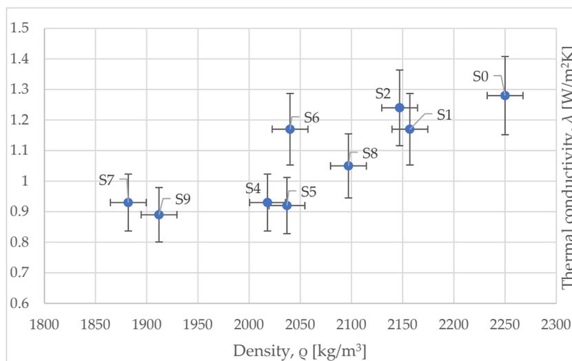
Figure 11. Variation of thermal conductivity versus density.
