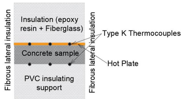
Figure 9. Experimental device.
