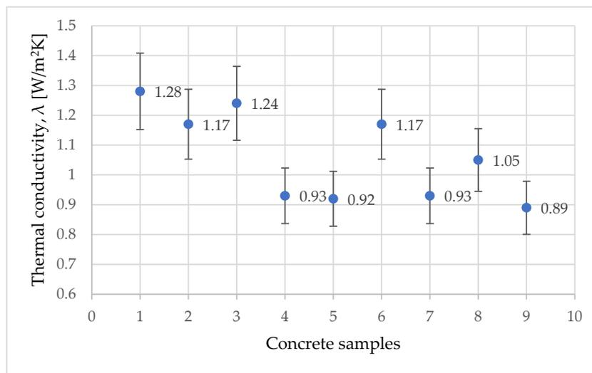
Figure 10. Variation of thermal conductivity.
