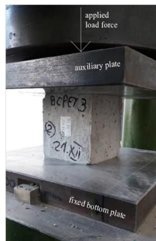
**Figure 5.** Experimental test of the compressive strength.
