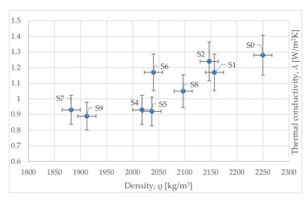
Figure 11. Variation of thermal conductivity versus density.
