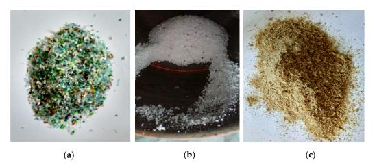
**Figure 3.** Waste aggregates used in the concrete mixture: (a) chopped PET bottle; (b) granular polystyrene; (c) sawdust/waste wood.
