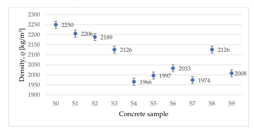
**Figure 6.** Variation of density for tested concrete samples.
