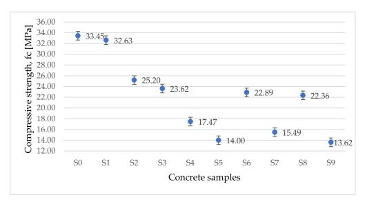
Figure 7. Variation of compressive strength for tested concrete samples.
