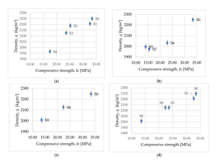
**Figure 8.** Variation of density versus compressive strength for concrete with waste: (a) concrete with waste chopped PET; (b) concrete with granular polystyrene; (c) concrete with sawdust; (d) concrete with waste chopped PET and sawdust.
