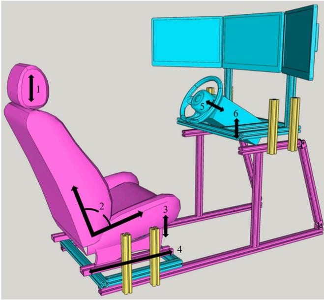
**Fig. 3.** Model of the static simulator (a). Black arrows represent the different mechanical adjustments possible on the simulator (1. Head-support height; 2. Backrest inclination; 3. Seat height; 4. Fore-aft adjustment of the seat; 5. Steering wheel fore-aft; 6. Steering wheel height). Picture of the simulator (b).
