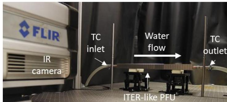
**Figure 2.** Picture of the ITER-like PFU emissivity testbed.
