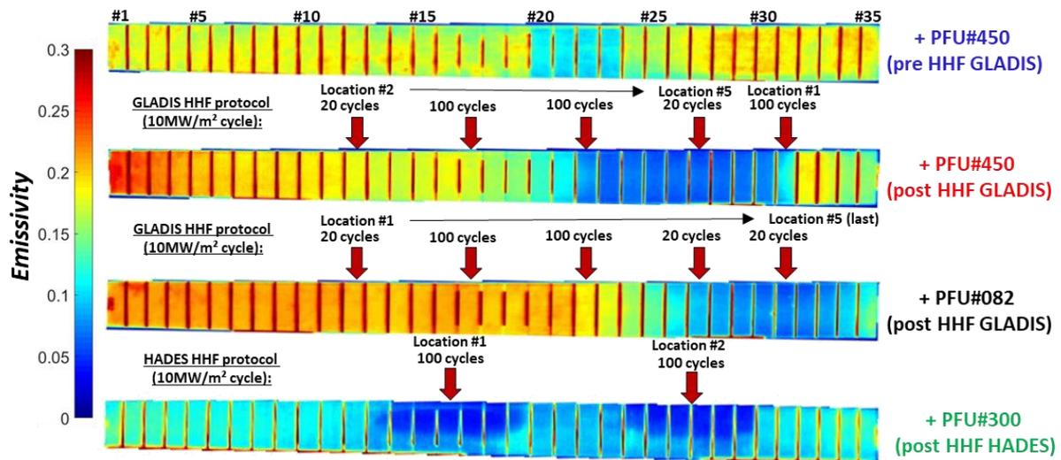
**Figure 4.** Emissivity map before and after high heat flux (HHF) tests for the PFU #450 and after HHF for PFU#082 performed at GLADIS and PFU#300 after HHF performed at HADES. Heat load location and order are indicated by red arrows. At each location about 5MB are exposed.
