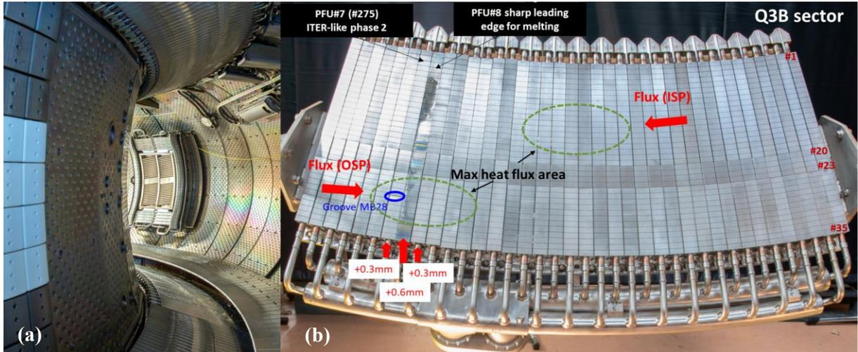
**Figure 1.** (a) Picture of WEST before the C5 experimental campaign. (b) Picture of the Q3B sector equipped with 35 bevelled ITER-like PFU and one unshaped ITER-like PFU (PFU#8). Vertical misalignments are indicated (red) as well as plasma direction (black) and maximum heat load location due to the ripple modulation (green dotted circle)
