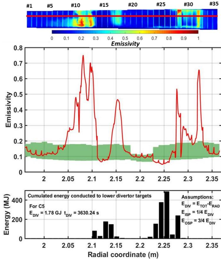
**Figure 6.** (Top) Emissivity map of the ITER-like phase 2 PFU #7 from the sector Q3B after C5. (Middle) Emissivity distribution along the lower divertor in red and green area corresponds to the emissivity dispersion observed for the 24 measured PFUs shown in figure 3. (Bottom) Conducted energy during C5 to the lower divertor at the strike point location with asymmetry of 1/4 ISP and 3/4 OSP as observed in [27] and no consideration of decay length ( $\lambda_q$ ).
