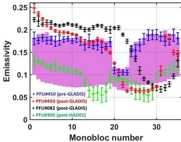
**Figure 5.** Average emissivity for each monobloc with distribution interval before and after high heat flux (HHF) test for the PFU #450 (blue and red) and after HHF for PFU#082 (black) performed at GLADIS and PFU#300 (green) after HHF performed at HADES. The purple area corresponds to the emissivity dispersion observed for the 24 measured PFUs shown in figure 3b.
