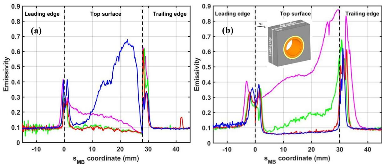
**Figure 8.** Emissivity of PFU #7 after C5 measured in the MB center along the curvilinear abscissa  $s_{MB}$  with  $s_{MB} = 0$  mm at the junction between the leading-edge and the top surface. (a) Inner strike point MB (blue) #13, (red) #14, (green) #15 and (magenta) #16. (b) Outer strike point MB (blue) #25, (red) #26, (green) #27 and (magenta) #28 inside the groove.
