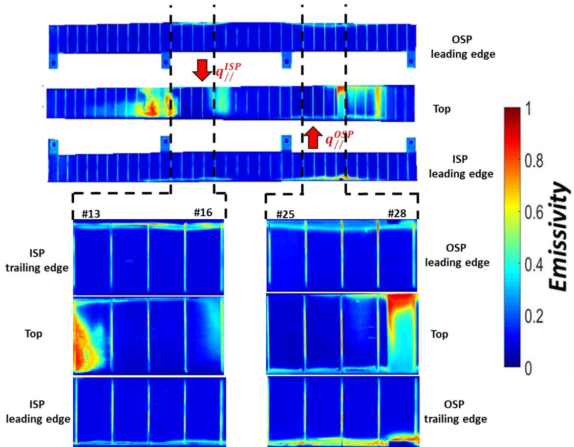
**Figure 7.** Emissivity map of the PFU #7 after C5. (top) Full PFU with top and lateral sides with 25 mm lens (0.7mm/pixel, full length analyzed of 437mm). (bottom) Zoom in for 4 MBs at the inner (left) and outer (right) strike point locations with 50 mm lens (0.08mm/pixel, full length analyzed about 50mm).
