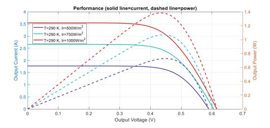
Figure 9: Evolution of the cell performance according to the variation of effective irradiance  $(500W/m^2, 750W/m^2)$  and  $1000W/m^2$ . The ambient temperature and exposed surface are considered constant:  $290^{\circ}K$  for the ambient temperature and  $0.01m^2$  for the surface.
