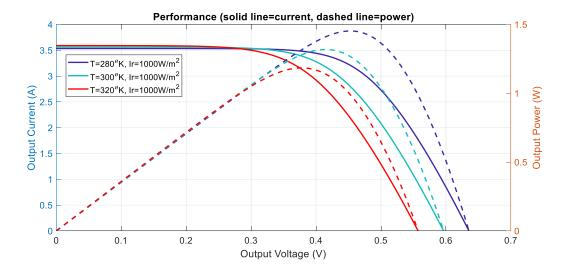
Figure 10: Evolution of the cell performance according to the variation of ambient temperature  $(280^{\circ}K, 300^{\circ}K \text{ and } 320^{\circ}K)$ . The irradiance and the exposed surface are considered constant:  $1000W/m^2$  for the irradiance and  $0.01m^2$  for the area.
