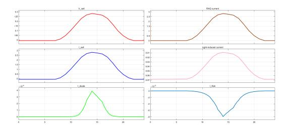
Figure 8: Evolution of the cell voltage  $v_{cell}$  and the cell current  $i_{cell}$ , the diode current  $i_D$ , the current passing through the resistance  $i_R$  of the electrical part of the system, the  $RAG_{current}$  and the light-induced current according to the variation of ambient temperature and irradiance.
