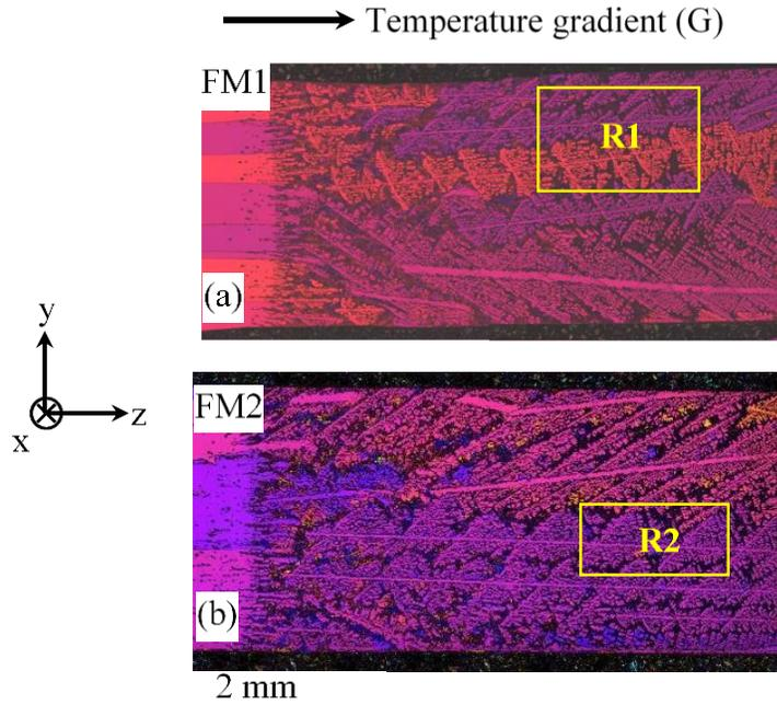
*Figure 1: Solidification microstructures obtained with optical microscope for FM1 and FM2 experiments solidified during the stage I. The yellow frames (boxes) indicate the regions of three-dimensional analysis. The solidification direction and the temperature gradient is along z direction.*
