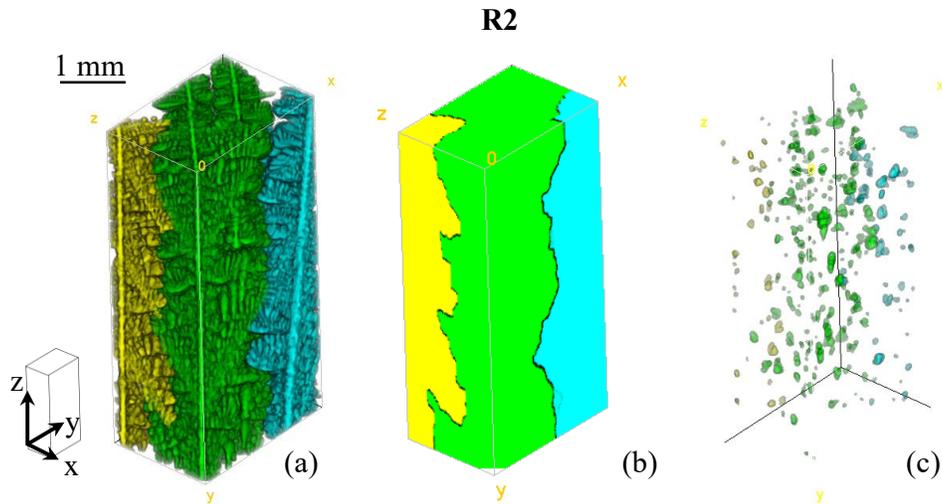
Figure 4: Image showing (a) the three dendrite groups in the R2, (b) their envelopes and (c) their corresponding fragments (according to colors).
