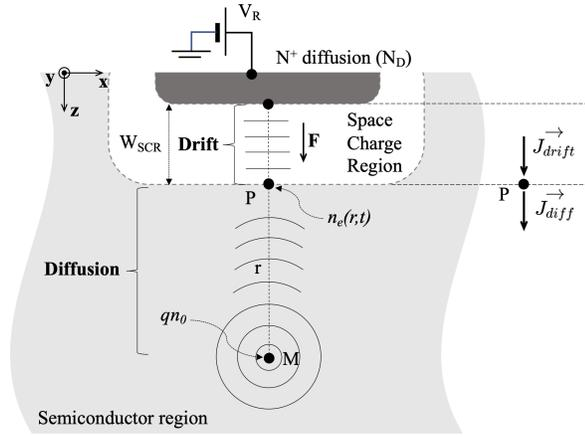
FIG. 9. Schematic illustration of the diffusion from a point charge and the collection by a reverse-biased  $N^+P$  junction.
