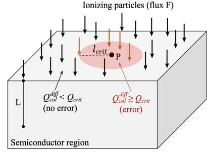
FIG. 5. Illustration of the concepts of critical distance  $l_{crit}$  and critical charge  $Q_{crit}$ . Any particle (characterized by the ratio  $N/L$ ) that impacts the disk centered in P and of radius  $l_{crit}$  will result in a collected charge above  $Q_{crit}$ , then inducing a soft error.
