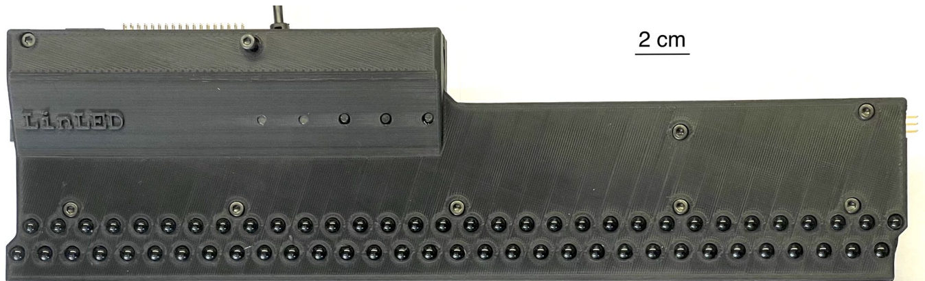
Figure 1: The patented LinLED interface composed of 32 near infrared photodiodes and 32 LEDs arranged along a 1D array. A finger or a hand moving in the air above LinLED at a height up to 40 cm can be located with an accuracy as small as 1 mm and a latency as fast as 1 ms.
