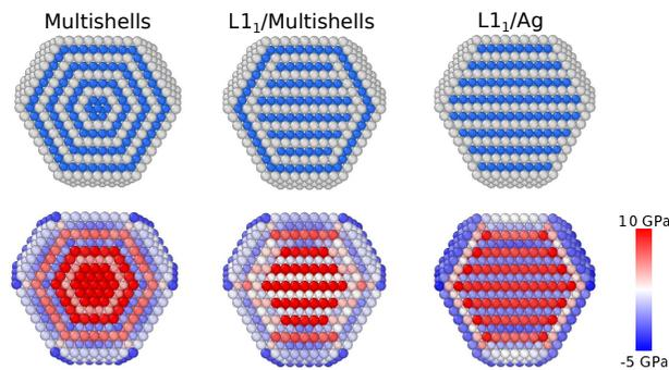
**Fig. 5** Cutting view of the 2951 atoms TOh with in top row the nature of the atoms (Ag in grey, Pt in blue) and in bottom row the stress map with color code corresponding to sites in compression in red (up to 10 GPa) and sites in tension in blue (up to -5 GPa).
