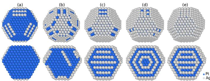
**Fig. 2** Snapshots of the  $\text{TOh}_{1289}$  at 200 K corresponding to the compositions pointed in Fig.1: (a) 7% of Ag, (b) 34% of Ag, (c) 54% of Ag, (d) 61% of Ag and (e) 65% of Ag. The top row represents the external surface whereas the bottom row displays a cutting view. Ag atoms are in grey and Pt atoms in blue
