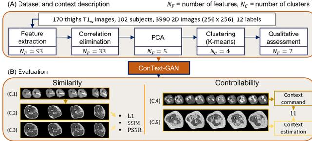
**Fig. 2.** A) Feature selection for context description. B) Evaluation process. C.1) Feature maps with same context, different topology. C.2), C.3) Generated and reference MRIs. C.4) Feature maps with same topology, different context. C.5) Generated MRIs from C.4). (Best zoomed)
