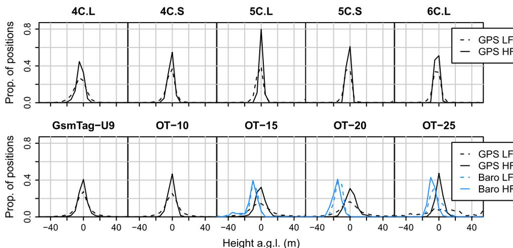
**Fig. 1** Distributions of the recorded heights above ground level from stationary positions on the ground for each tag model and method. The lines connect the proportions of positions per height class of 5 m (central class centred around zero). Height data < − 50 and > 50 m a.g.l. not shown. *Prop.* proportion, *LF* low frequency, *HF* high frequency
