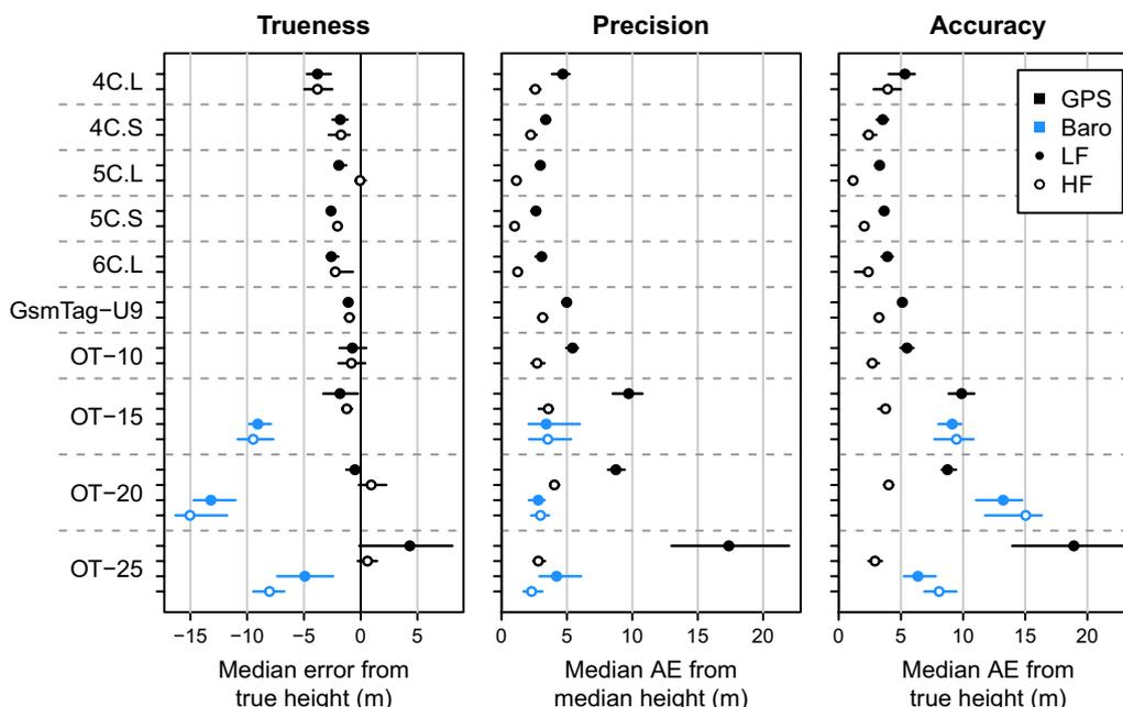
**Fig. 2** Estimates and 95% confidence intervals for trueness, precision and accuracy for each combination of GPS tag model and method based on hierarchical bootstrapping. Parameters used: median error with true height as reference (equivalent to median height a.g.l.; trueness), median absolute error with median height as reference (precision), median absolute error with true height as reference (accuracy). *a.g.l.* above ground level, *AE* absolute error
