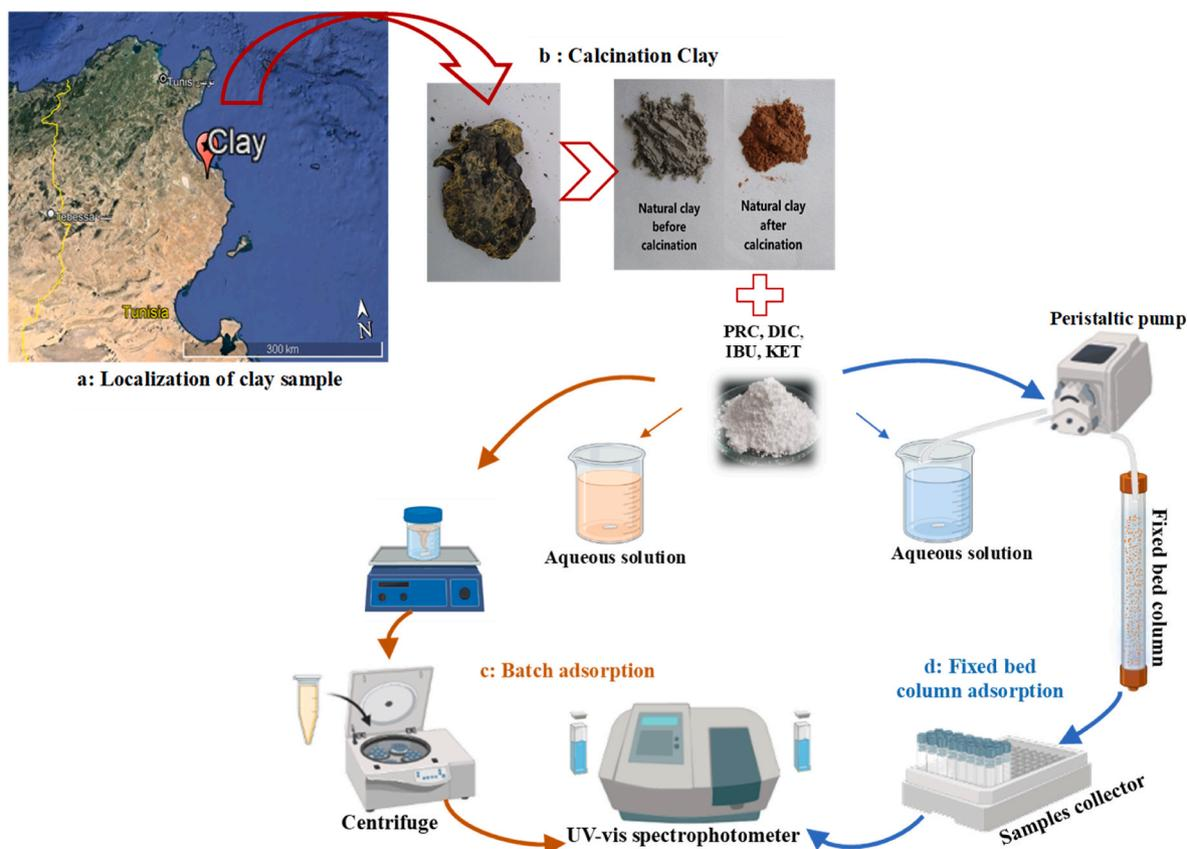
Fig. 1. (a) Localization of clay sample collected from the region of ZBH; (b) Clay adsorbent after calcination at 550 °C; (c) Batch adsorption experiments; (d) Fixed bed column adsorption experiments.
