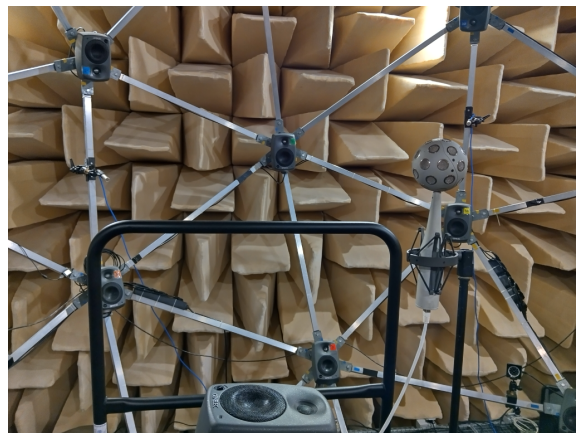
Figure 3: Evaluation setup composed of control loudspeaker Genelec 8020 and a control microphone mh acoustics em 32 (for the multichannel evaluation).
