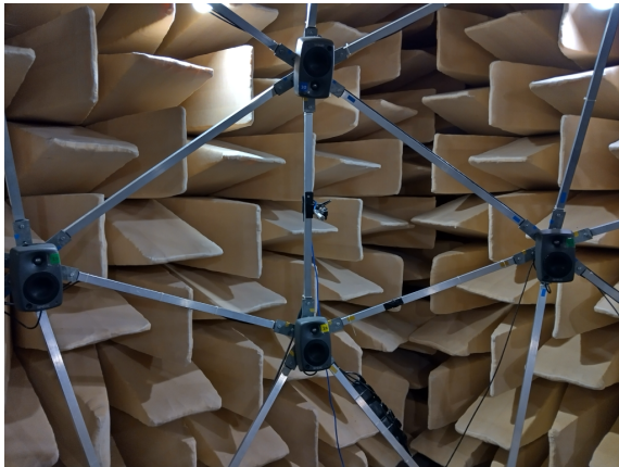
Figure 1: Part of the 42-loudspeakers spherical array, and auralization microphone on the center.
