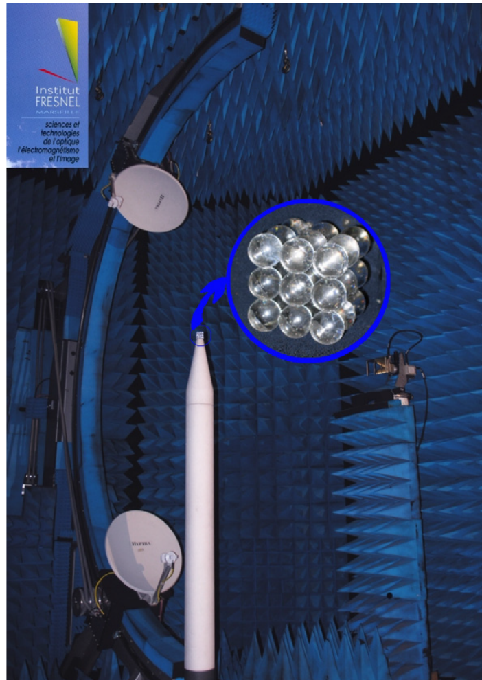
FIGURE 5.14 – Picture of the anechoic chamber at the Center Commun de Ressources Micro-Ondes (CCRM) which was used to measure the scattered field data of different targets of the Fresnel database.
