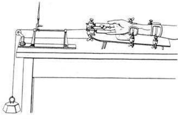
**Fig. 20 The classical finger ergograph developed by Mosso (1892)**
