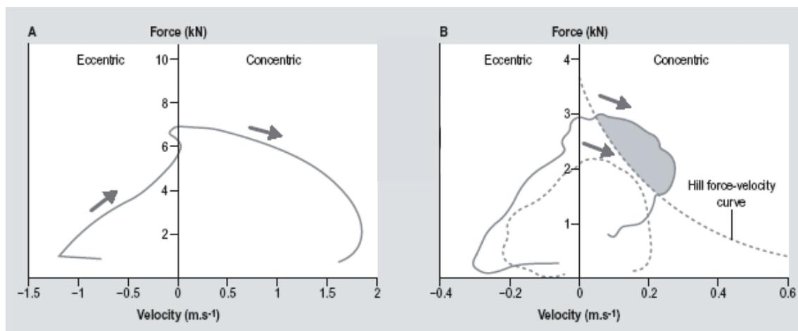
**Fig. 7. Instantaneous force-velocity (F-V) curves.** F-V curves measured with a buckle transducer on the Achilles tendon during running (A:  $9 \text{ m.s}^{-1}$ ), and with an optic fibre for the Achilles (solid) and patella tendons (dashed) during hopping (B). Note the force potentiation during the concentric phase of the stretch-shortening cycle (shaded area). (Adapted from Komi 1992 (A) and Finni et al. 1998 (B))
