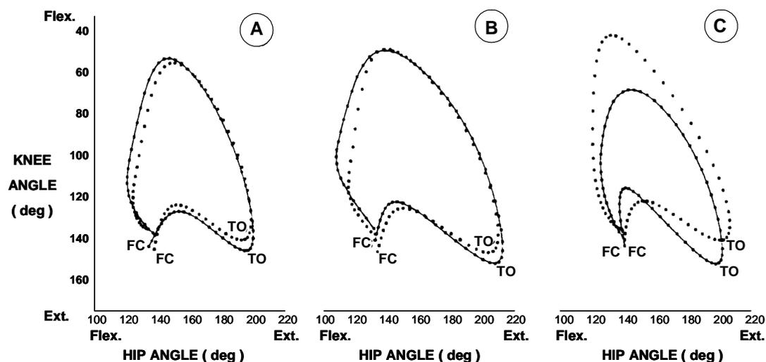
**Fig. 66.** Examples (subjects A, B and C) of hip-knee angle cyclograms measured before (cut line) and after (black line) the marathon at the fast ( $4.5\text{-}6\text{ m}\cdot\text{s}^{-1}$ ) treadmill running speed. (Adapted from Nicol et al. 1991a)
