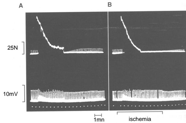
**Fig. 22.** (A) A maximal voluntary effort persisted until severely fatigued. A series of single twitches precede and follow. Lower trace, the corresponding action potentials. Time markers ½ min. (B). The same but with the circulation occluded for the period indicated by a line beneath the record. (From Merton 1954)
