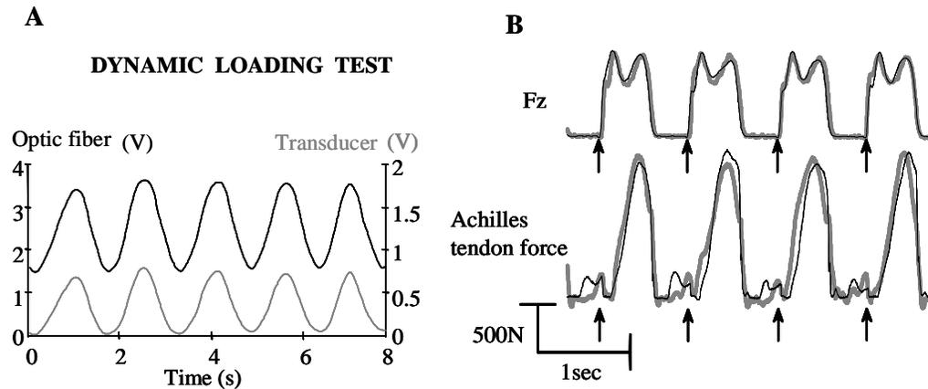
**Fig. 6. Optic fiber recordings in dynamic testing conditions.**
