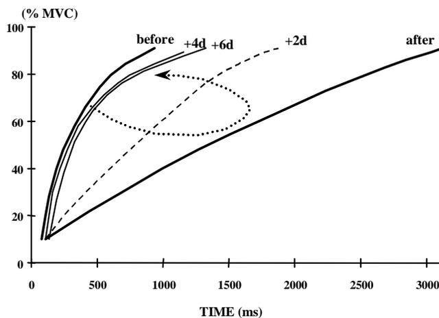
**Fig. 50:** Isometric force-time curves of the maximal knee extension measured immediately before and after a marathon run as well as 2, 4 and 6 days later. Note the large and immediate decrease in the rate of force development and its slow recovery towards the 4th day post-marathon. (Data from Pullinen et al. 1999)
