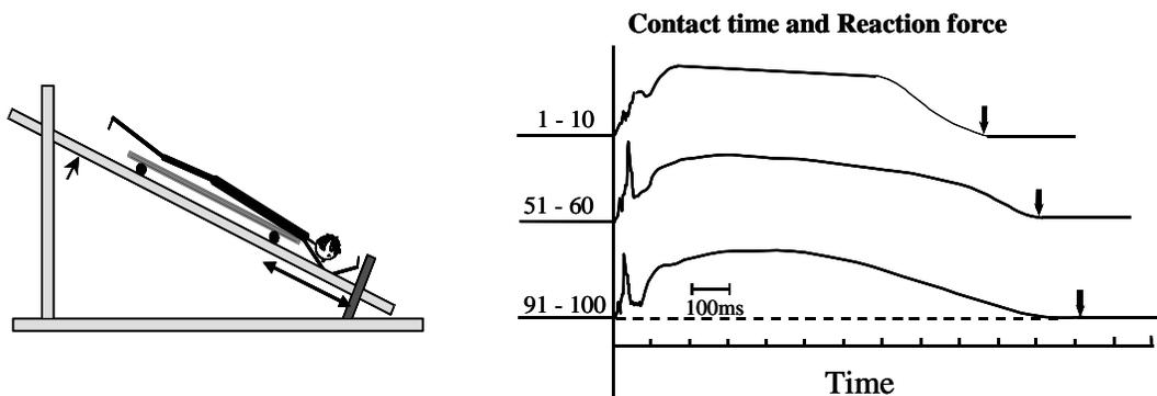
**Fig. 43. Relative changes in kinetics (contact time and reaction force) during the time course of 100 submaximal rebounds with the upper limbs.** (Data from Gollhofer et al. 1987b)
