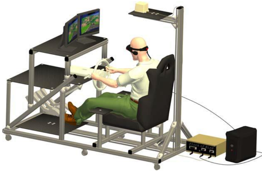
Figure 21: Overview of the set-up. Participants sat on a play seat integrated into an aluminum frame and wore a head mounted display. They controlled the velocity of the virtual car with accelerator and brake pedals and lateral excursions between lanes with the steering wheel. Participants' head pitch, yaw and roll orientations were measured with an electromagnetic tracker and coupled to the visual scene. Participants could also display rear mirrors by pressing buttons on the steering wheel.
