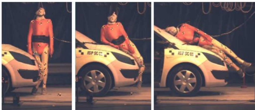
Figure 9: Example of pedestrian crash on a vehicle from Masson et al. (2007)
