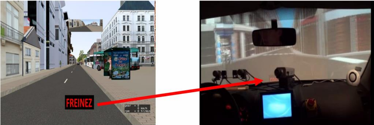
Figure 117: Visual display of FCW signal on the simulator screen and from passenger seat point of view
