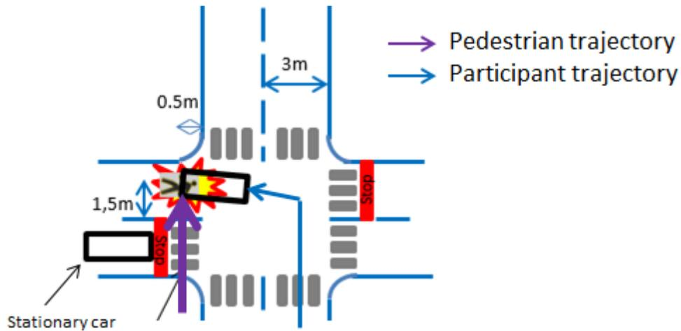
Figure 105: Turning Left and Pedestrian Left configuration
