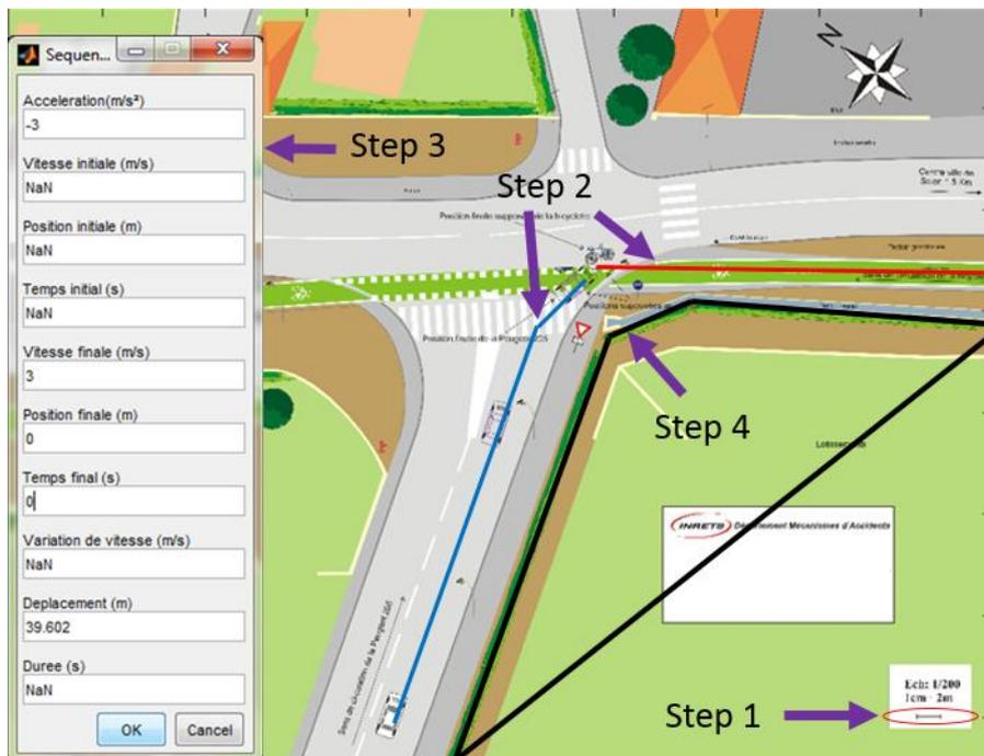
Figure 11: Accident kinematic reconstruction method
