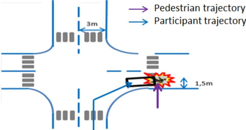
Figure 109: Turning Right and Pedestrian Right configuration
