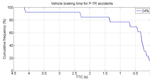
Figure 31: Drivers' braking timing for the P-TR scenario, 24% braking activation among 55 P-TR accident cases
