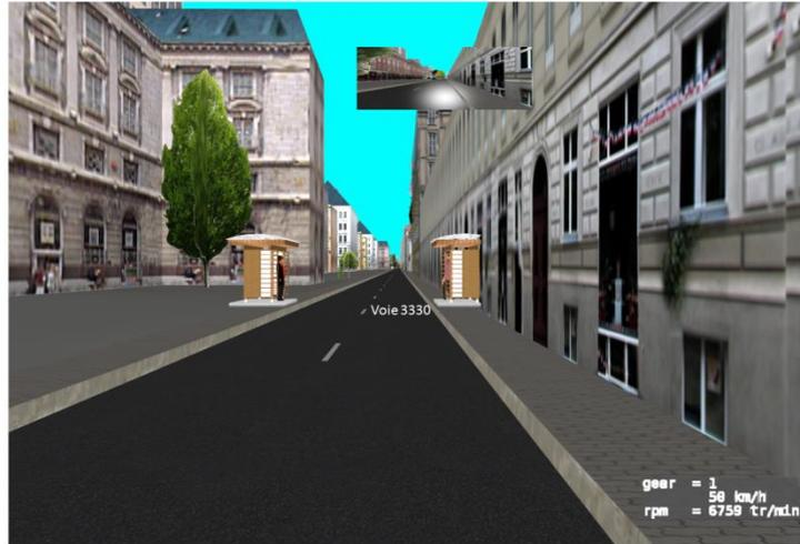
Figure 1: pattern of the Pedestrian Crossing Nearside scenario on the left side of the figure. The trigger of the Pedestrian is based on vehicle instant speed 2.5s before the vehicle center arrives to the position of the Pedestrian. On the right side of the figure, the lateral position from where the Pedestrian becomes visible.
