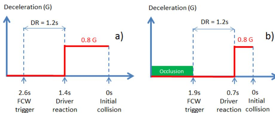
Figure 135: FCW trigger model in the simulation
