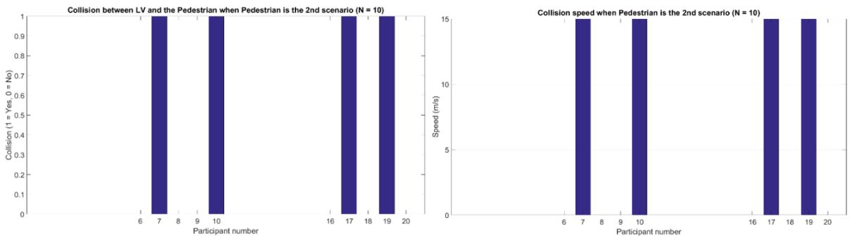
Figure 21: Results when Pedestrian CN is the 2nd scenario. Number of collisions (4 out of 10) on the left and collision speed of the right. Mean value and standard deviation: 15 (0). Min value: 15 and max value: 15.
