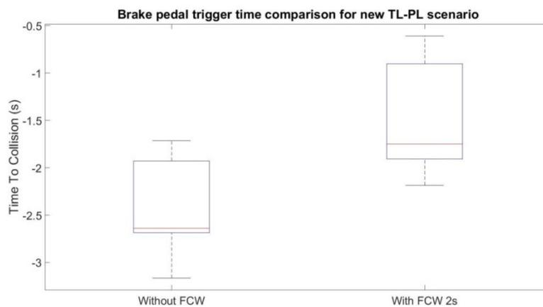
Figure 132: Brake trigger time for new TL-PL scenario
