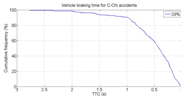
Figure 35: Drivers' braking timing for the C-CN scenario, 29% braking activation among 744 C-CN accident cases
