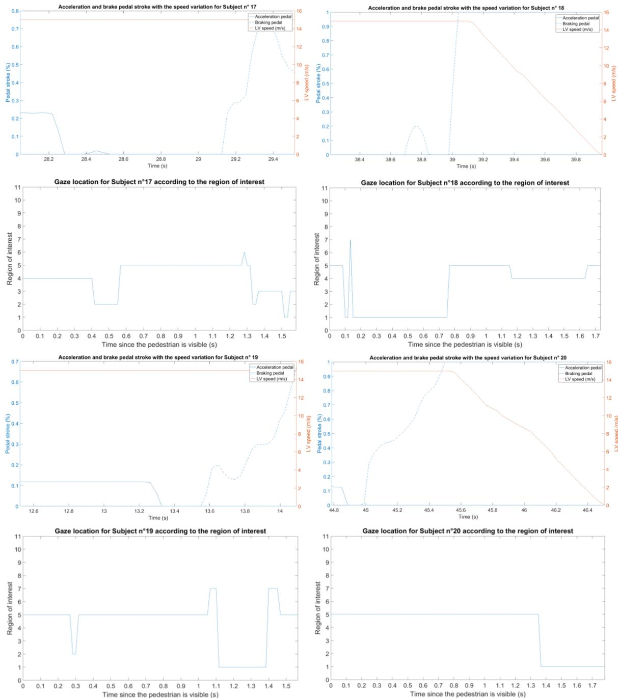
There is statistically no difference between participants from the first moment they activate the brakes. Most participants seem to have seen the pedestrian crossing as brakes have been triggered. Current analysis is not precise enough to determine exactly what can be perceived as only a region of interest can be determined here. An improvement for gaze analysis can be obtained with the gaze position in the driving simulator environment as described in the conclusion section.
