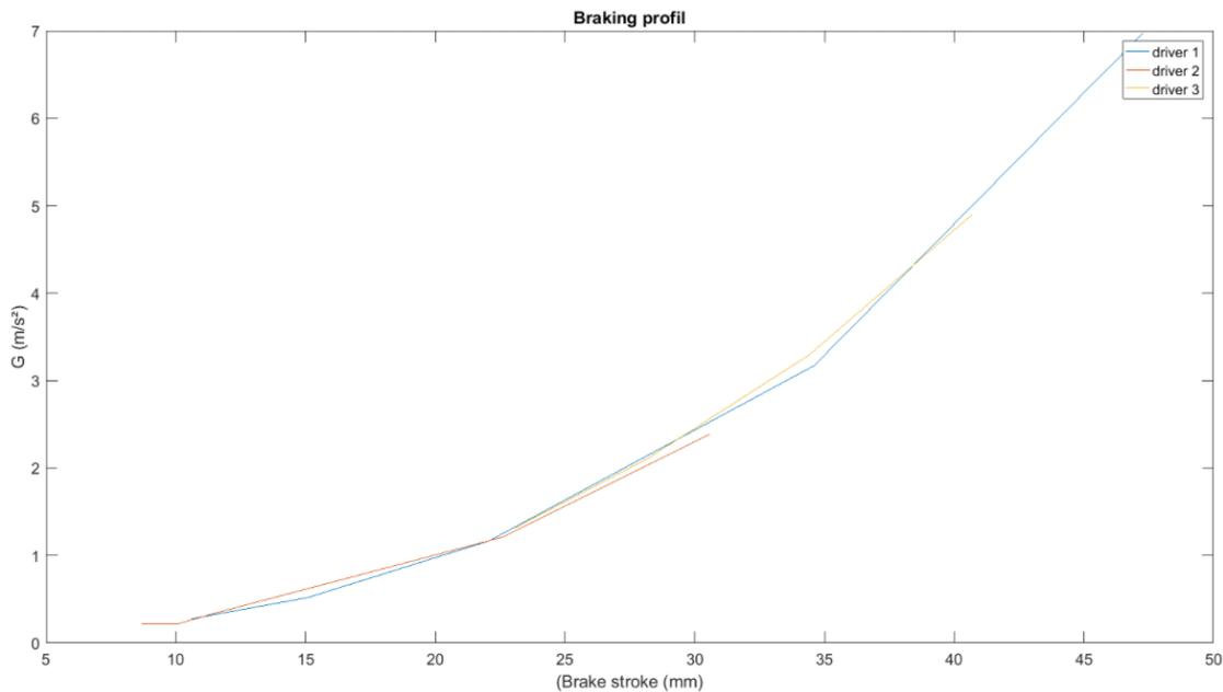
Figure 100: Brake deceleration profile of the driving simulator
