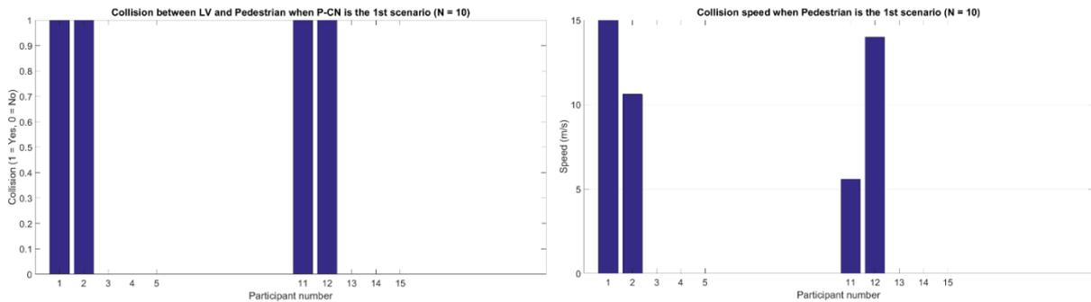
Figure 20: Results when Pedestrian CN is the 1st scenario. Number of collisions (4 out of 10) on the left and collision speed on the right. Mean value and standard deviation: 11.2955 (4.2420). Min value: 5.5900 and max value: 15.
