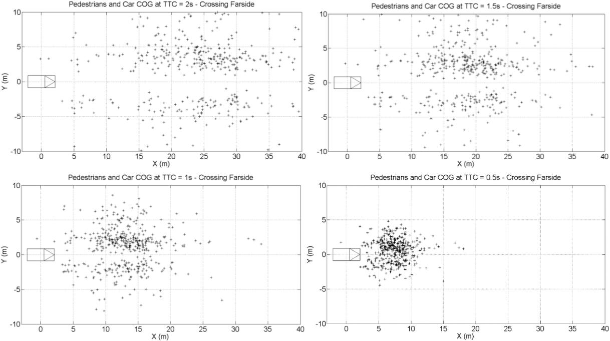
Figure 24: Pedestrians' positions relative to the vehicle 2s, 1.5s, 1s and 0.5s before the impact for all P-CF accidents (N = 461)
