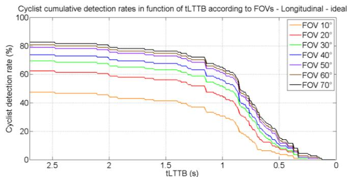
Figure 77: Detection rates at  $t_{LTTB}$  for different FOV for the cyclist longitudinal scenario,  $N = 120$
