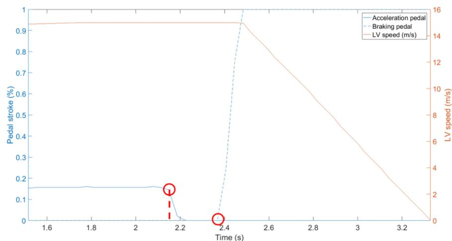
Figure 118: Gas and brake pedal time extraction
