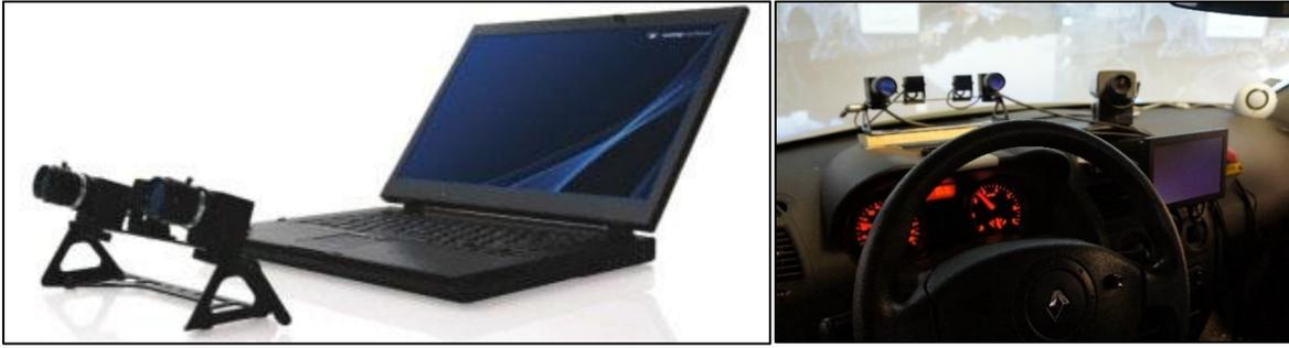
Figure 98: Facelab eye tracking device
