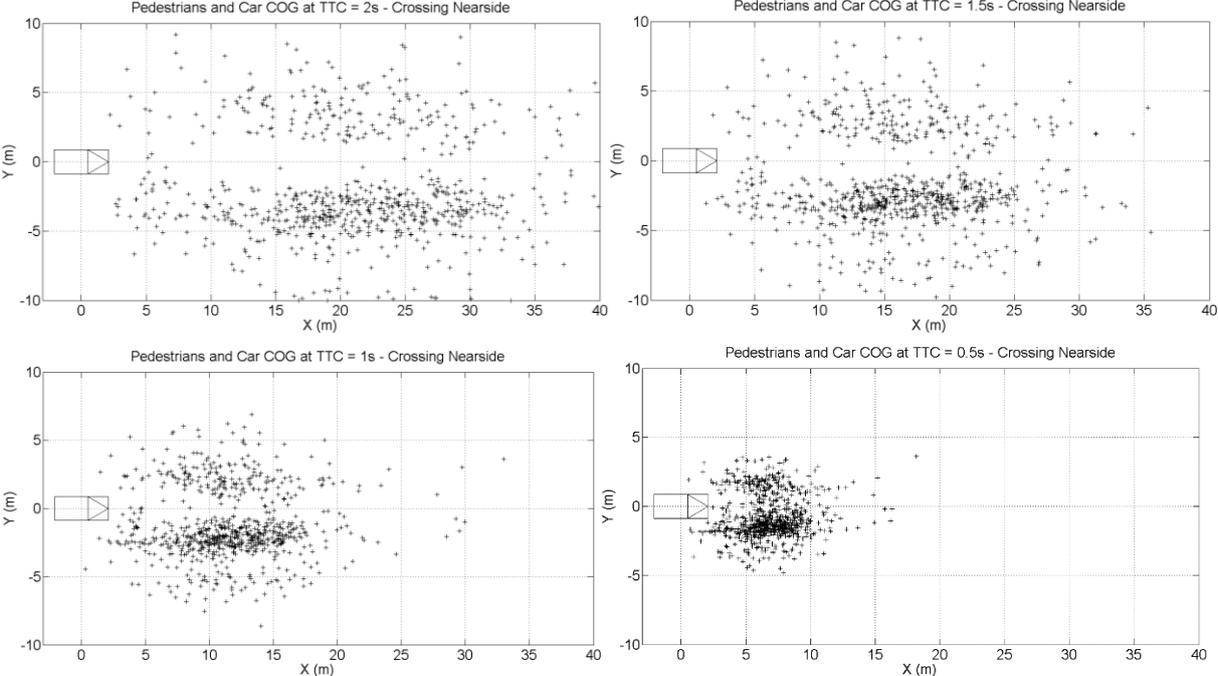
Figure 22: Pedestrians' positions relative to the vehicle 2s, 1.5s, 1s and 0.5s before the impact for all P-CN accidents (N = 788)
