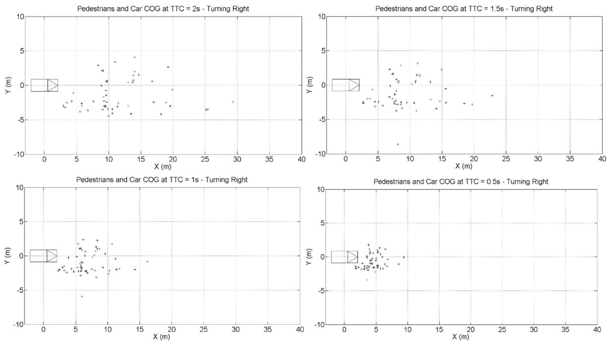
Figure 30: Pedestrians' positions relative to the vehicle 2s, 1.5s, 1s and 0.5s before the impact for all P-TR accidents (N = 55)
