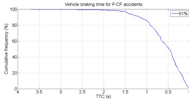
Figure 25: Drivers' braking timing for the P-CF scenario, 61% braking activation among 461 P-CF accident cases
