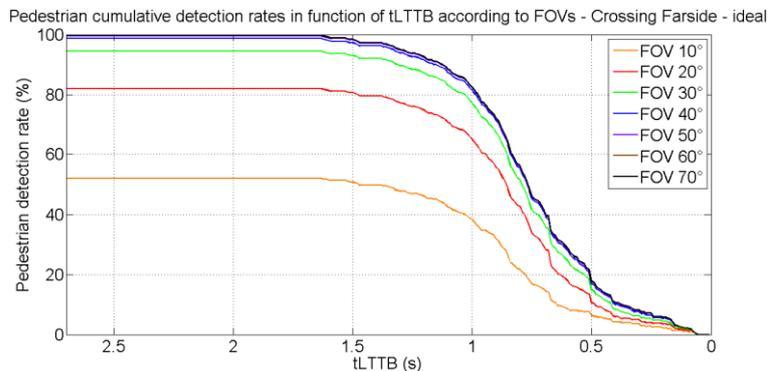
Figure 70: Detection rates at  $t_{LTTB}$  for different FOV for the pedestrian crossing farside scenario, N = 461
