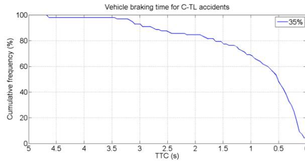
Figure 41: Drivers’ braking timing for the C-TL scenario, 35% braking activation among 280 C-TL accident cases
