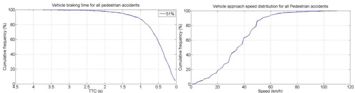
Figure 21: (Left) Cumulative frequency of brake activation timing (51% of all cases) and vehicle approach speed (Right), N = 1509
