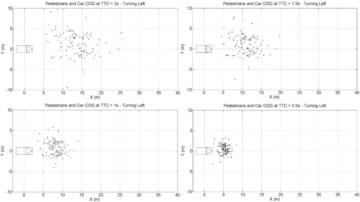
Figure 28: Pedestrians' positions relative to the vehicle 2s, 1.5s, 1s and 0.5s before the impact for all P-TL accidents (N = 124)
