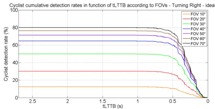
Figure 79: Detection rates at  $t_{LTTB}$  for different FOV for the cyclist turning right scenario,  $N = 492$
