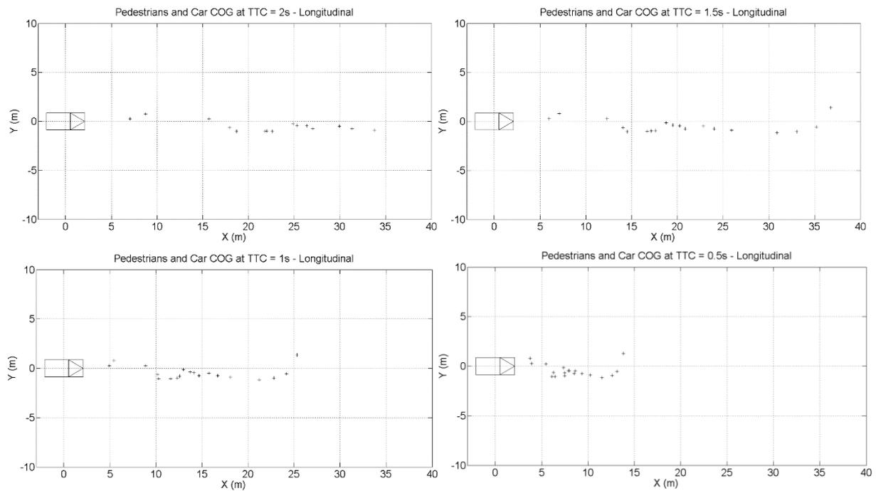
Figure 26: Pedestrians' positions relative to the vehicle 2s, 1.5s, 1s and 0.5s before the impact for all P-L accidents (N = 20)
