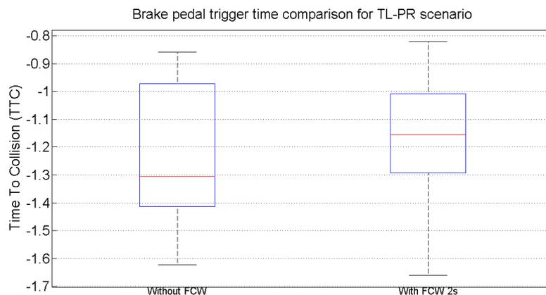
Figure 127: Brake trigger time boxplot for TL-PR scenario
