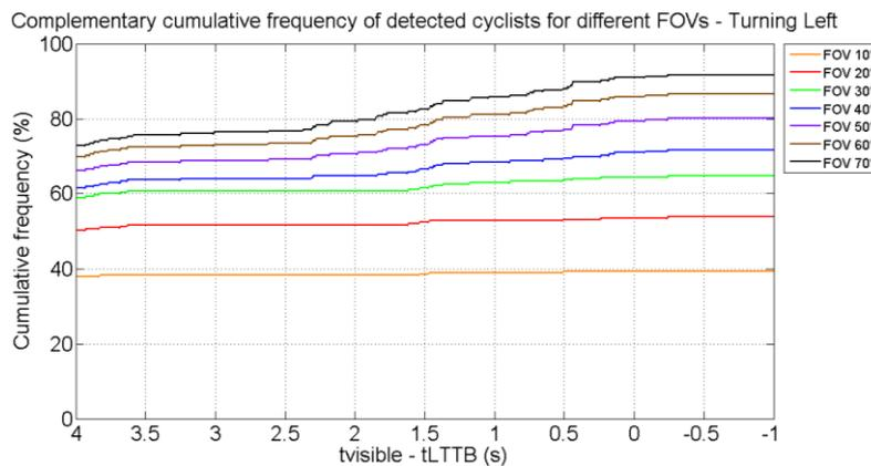
Figure 90: Detection rates at  $t_{\text{visible}} - t_{\text{LTTB}}$  for cyclist turning left cases,  $N = 280$
