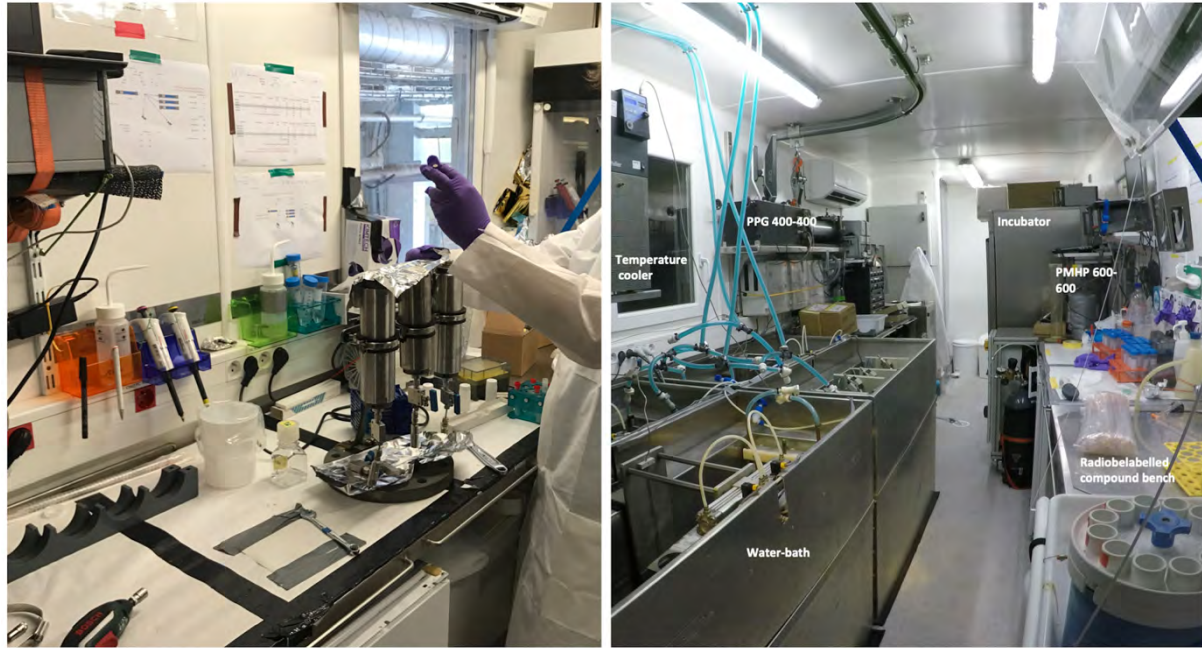
Supplementary Figure 2-3 Photograph showing different point of view of MIO-HPLab. This mobile laboratory has been constructed in a 20 feet container. It is composed of two piloted pressure generators, four temperature regulated water baths with two temperature coolers dedicated for HPSU and PASS experiments (Tamburini et al., 2009), and a reinforced Peltier-cooled incubator Memmert IPP 750 oven for HPBs incubation. The mobile laboratory (MIO-HPLab) is also certified to use radiolabeled during oceanographic cruises.
