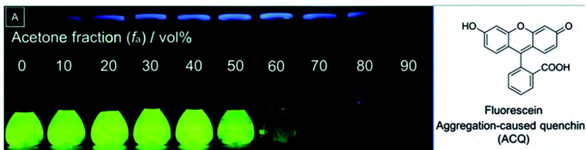
Figure 10: ACQ in fluorescein ( 15\mu\text{M} ) in water/acetone mixture with different fractions of acetone ( f_a ). (Reprinted with permission). [97]
