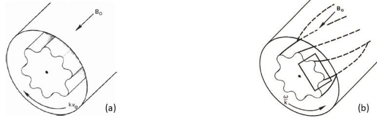
Figure 3.2.: (a). Flute mode with k_{\parallel} = 0 (Source [Che16]) (b). Screw mode with k_{\parallel} > 0 (Source [Che16]).
